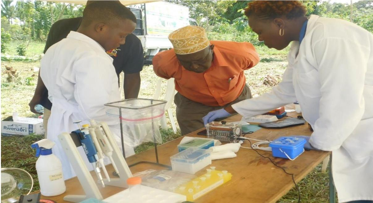
*A field trial of Mini – mobile PCR machine to reduce the time between sample collection and result dissemination to the farmers.*
